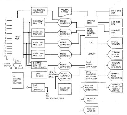
Fig. 3 Hardware block diagram.
